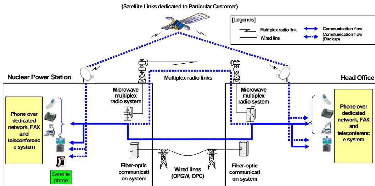
**Fig. 3-2 Overview of Telecommunications Facilities inside Kyushu EPCO for Communications outside Power Stations**
