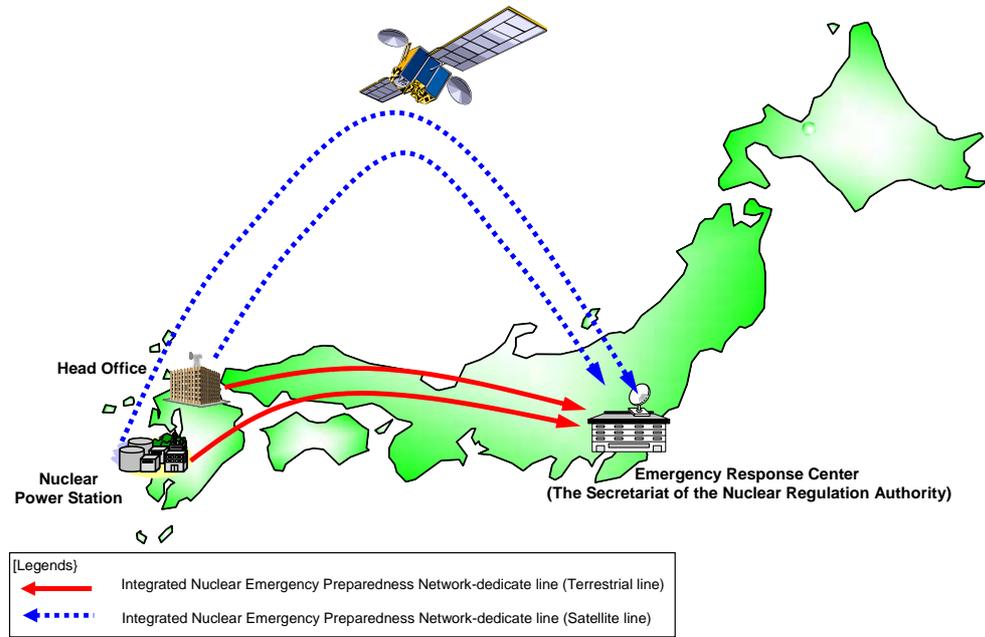
**Fig. 3-3 Overview of Telecommunications Facilities outside Kyushu EPCO for Communications outside Power Stations**
