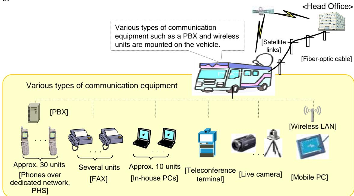
**Fig. 3-5 Overview of Emergency Communications Vehicle**
