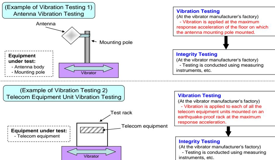
**Fig. 3-4 Overview of Vibration Testing**
