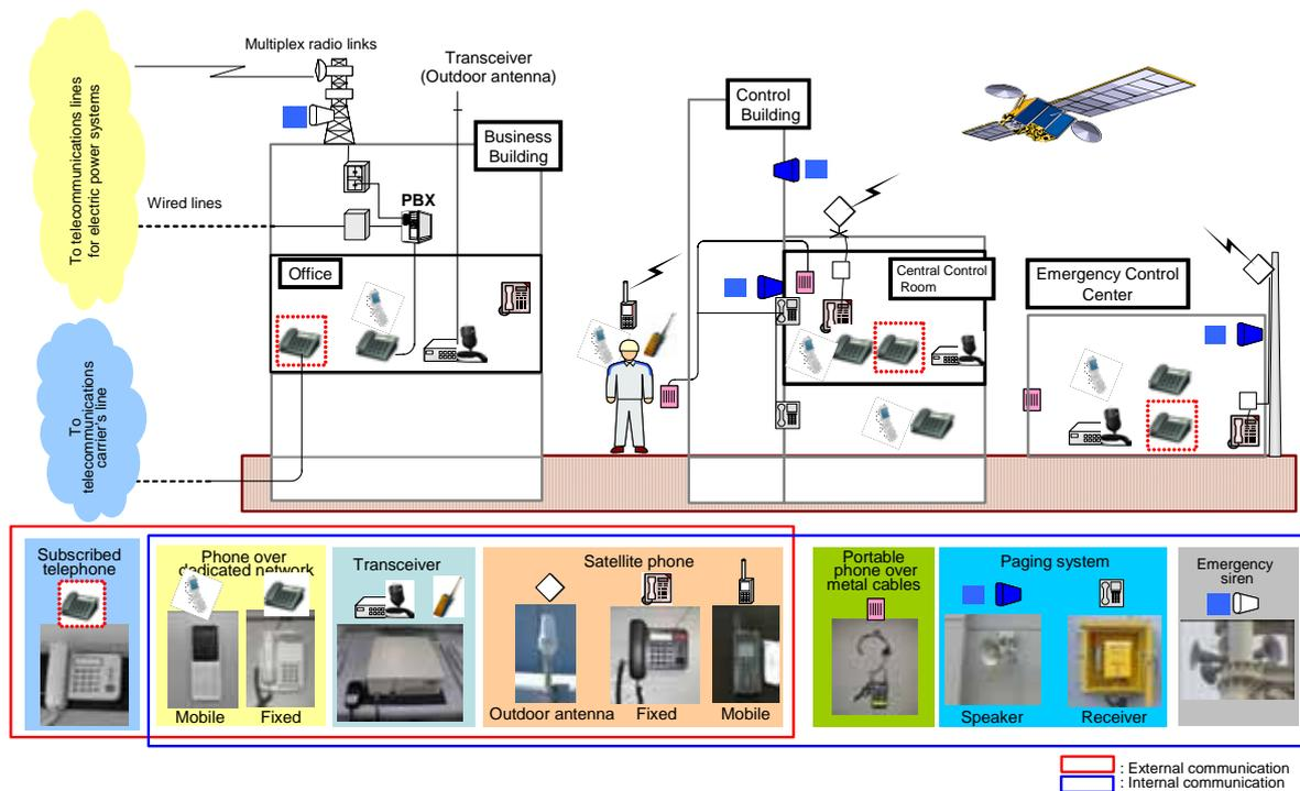
**Fig. 3-1 Overview of Telecommunications Facilities for Communications inside Power Stations**
