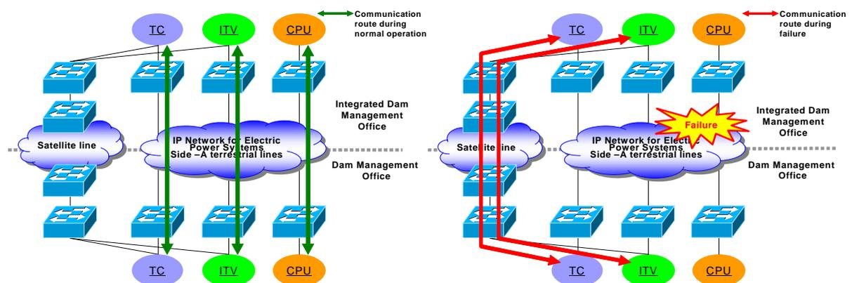
**Fig. 2-2 Communication Routes using Terrestrial Lines during Normal Operation and Satellite Line as Backup**
