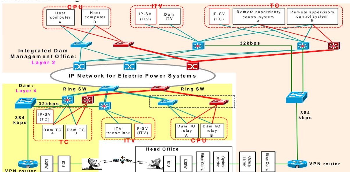
**Fig. 2-1 Configuration of Integrated Dam Management System and Network**
